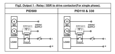
NOTE: Use snubber as shown above to increase life of internal relay of temperature controller.
