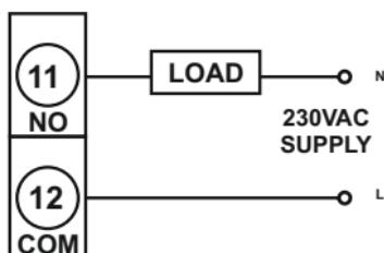
**Fig2. Output 1 - Relay / SSR to drive contactor(For single phase).****PID500**
