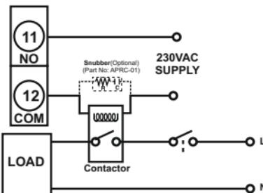
**NOTE:** Use snubber as shown above to increase life of internal relay of temperature controller.
