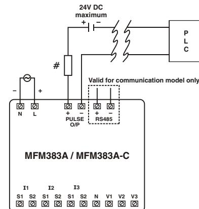
Pulse output from MFM383A meter can be interfaced into a process through a PLC for on line control of energy content in the process.
