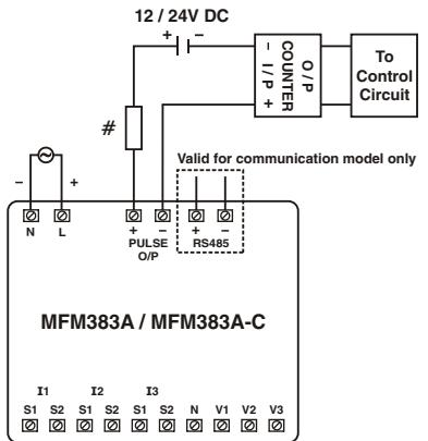
Pulse output from MFM383A meter can be used as alarm generator or total energy controller by interfacing it with Pre-settable counter and control circuits (Contactors, Relay, Trip Circuit).
