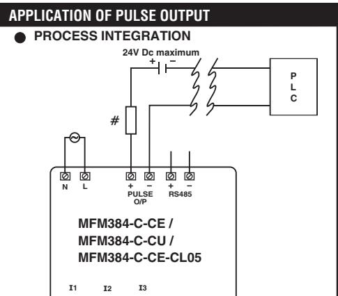
Pulse output from MFM384-C meter can be interfaced into a process through a PLC for on line control of energy content in the process.
