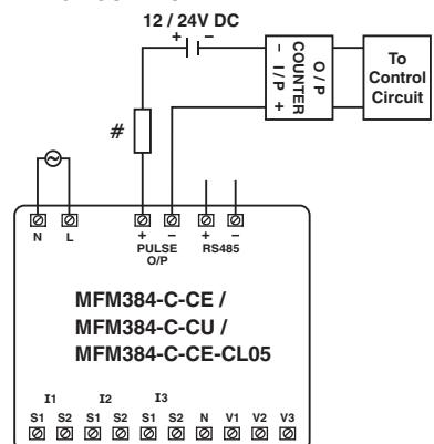
Pulse output from MFM384-C meter can be used as alarm generator or total energy controller by interfacing it with Pre-settable counter and control circuits (Contactors, Relay, Trip Circuit).
