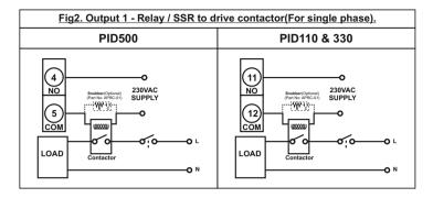
**NOTE:** Use snubber as shown above to increase life of internal relay of temperature controller.
