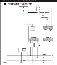
Pulse output from MRJ385-G-PNW meter can be interfaced into a process through a PLC for on line control of energy content in the process.
