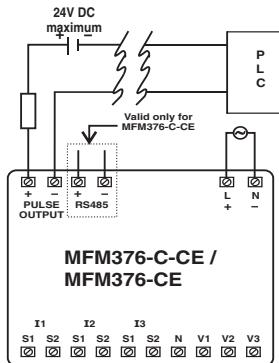
Pulse output from MFM376-C-CE / MFM376-CE meter can be interfaced into a process through a PLC for on line control of energy content in the process.
