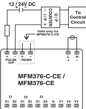
Pulse output from MFM376-C-CE / MFM376-CE meter can be used as alarm generator or total energy controller by interfacing it with Pre-settable counter and control circuits (Contactors, Relay, Trip Circuit).
