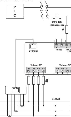
Pulse output from MRJ385-G-PNW meter can be interfaced into a process through a PLC for on line control of energy content in the process.
