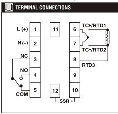
Use only the correct thermocouple wire or compensating cable from the probe to instrument terminals avoiding joints in the cable if possible. Failure to use the correct wire type will lead to inaccurate readings.
