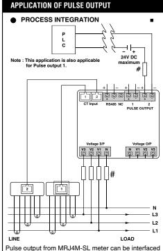
Pulse output from MRJ4M-SL meter can be interfaced into a process through a PLC for on line control of energy content in the process.
