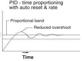
The PID values obtained are stored in the nonvolatile memory.
