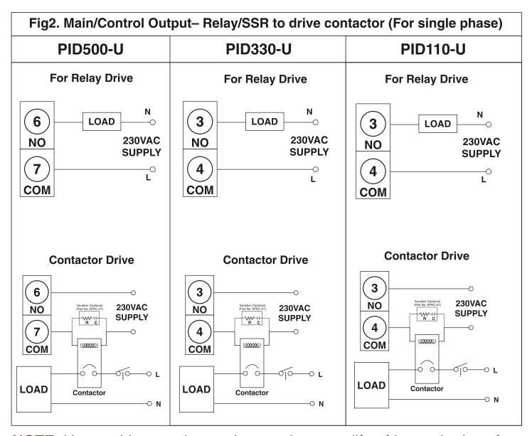
**NOTE**: Use snubber as shown above to increase life of internal relay of temperature controller.
