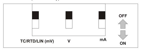
Push the respective switches downwards for hardware selection of Input sensor types.
