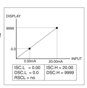
Reverse acting indication can be accomplished by setting **reverse scaling** parameter as YES. In this case **referring the above eg.** for 0.00 mA input the display will show 9999 and 20.00 mA input the display will show 0.0 **NOTE:** This change will not be visible in the programming menu.
