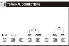
Use only the correct thermocouple wire or compensating cable from the probe to instrument terminals avoiding joints in the cable if possible. Failure to use the correct wire type will lead to inaccurate readings. Ensure that the input sensor connected at the terminals and the input type set in the temperature
