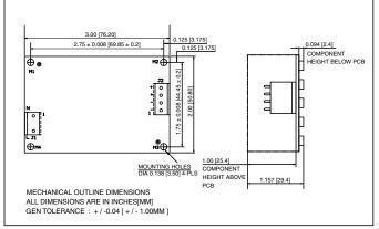
Note: 1. This open frame power supply should preferably be mounted horizontally on 4 metal
