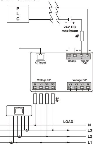
Pulse output from MRJ385-G-PNW meter can be interfaced into a process through a PLC for on line control of energy content in the process.
