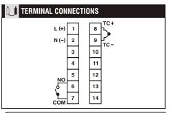
Use only the correct thermocouple wire or compensating cable from the probe to instrument terminals avoiding joints in the cable if possible. Failure to use the correct wire type will lead to inaccurate readings.
